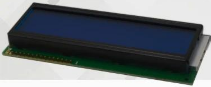
16x2 COB Character LCD Module
