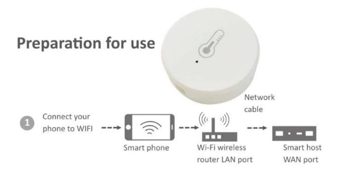
Make sure that the product is within the effective coverage of the smart host (gateway) Zigbee network to ensure the effective connection between the product and the smart host (gateway) Zigbee network.
